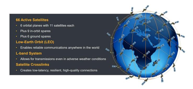
Iridium Certus runs on high-speed L-Band. L-Band is the lowest frequency commonly available for maritime satellite communications, meaning that the Iridium signal can penetrate clouds, fog, and rain better than higher frequency Ka-and Ku- band signals.
